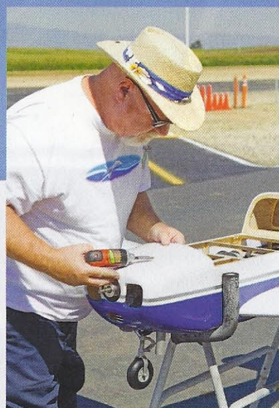
The reviewer installs the included Phillips head screws to the cowl with a power screwdriver.
