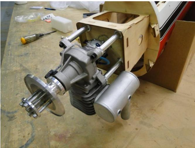
Top View of installed Engine.
