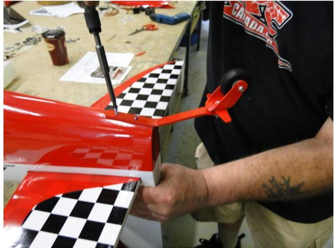
***TIP: Remove the screws and add a drop of Thin CA Glue to each hole and re-attach the Tail Wheel Bracket. This will help harden the Balsa and stop the Wood Screws from loosening.***
