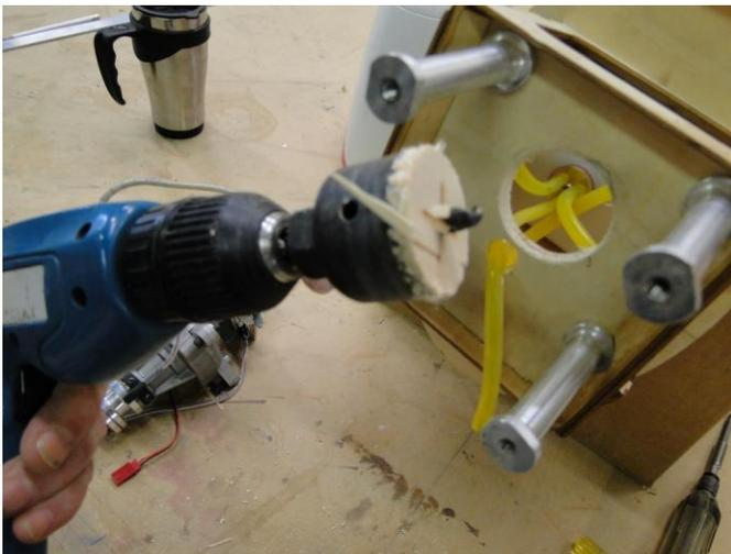
Use a hole saw to cut out a hole at least 1-1/4 diameter if you have a rear mounting carburetor (to breathe). It also allows passage of the Fuel Lines.
