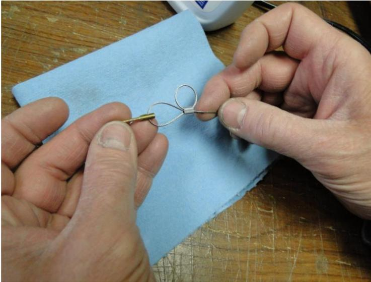
***TIP: An extra loop of the Cable through the Crimp Fitting will make the connection stronger.***
