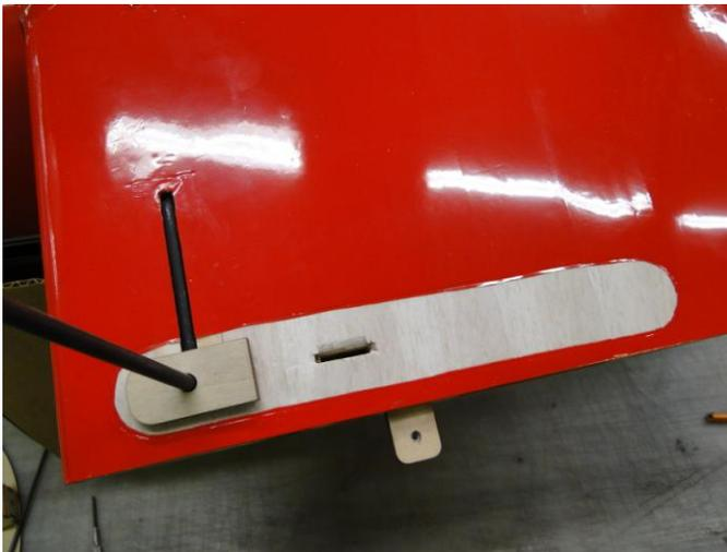
Use a sharp X-Acto Knife to carefully cut away the Covering about 1/16 inch inside the lines. Be careful not to cut into the Balsa.
