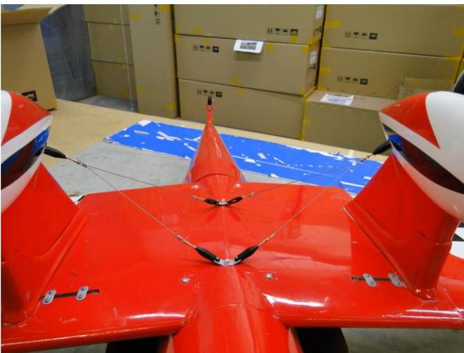
Repeat the same process for the Wires between the two Wheel Pants along the center line of the Middle Wing.
