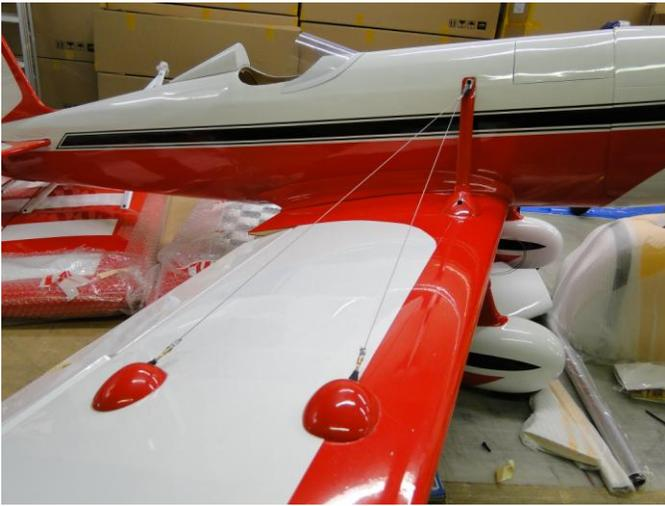
Repeat the same process for the Wires on the top of the Wing from where the Strut attaches to the Fuselage.
