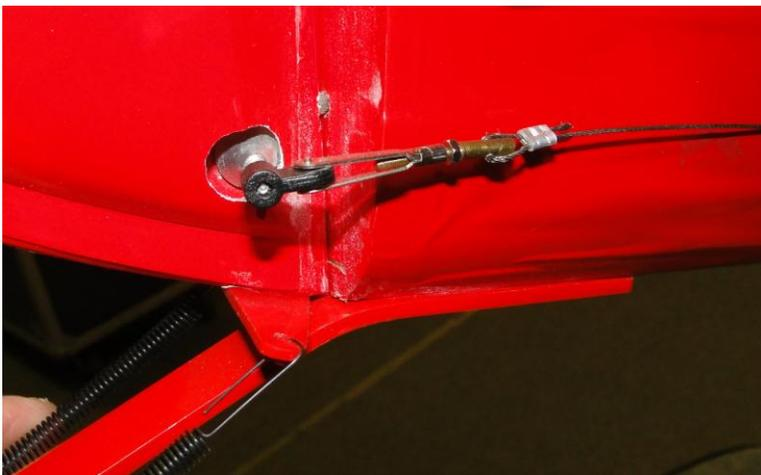
When satisfied with the lengths, carefully crimp the Cable fittings and trim the excess Cable.
