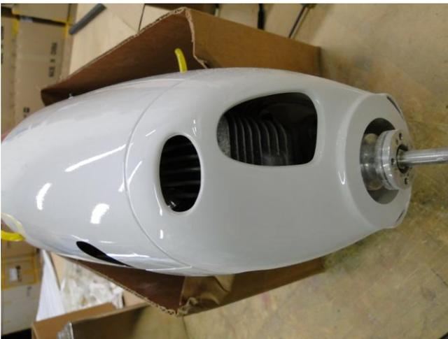
Also cut out necessary holes in the Cowl for the proper Engine cooling using a Dremel Tool.
