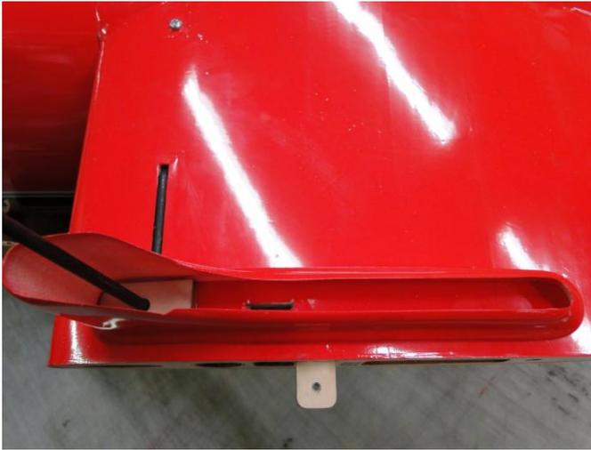
Use Epoxy to glue the lower Wheel Pant in place, pushed up against the Plywood Wheel Pant Insert.
