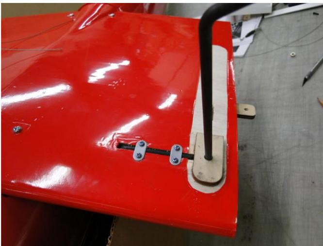
Attach the Straps using Screws supplied.
