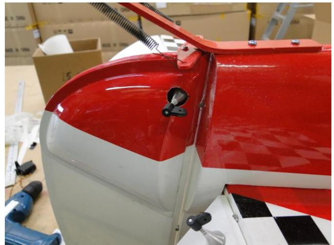
Cut the Cable into 2 equal lengths and thread the Cable through these new uncovered holes in the rear of the Fuselage. Thread one Crimp Fitting over the end of one Cable, then thread the Cable through the outer hole in the your Large Rudder Servo Arm. Fold back the Cable 1 inch and slide the Crimp Fitting over the Cable end. When satisfied with the fit, crimp the fitting. Repeat for the other end of the Servo Arm with the other Cable.
