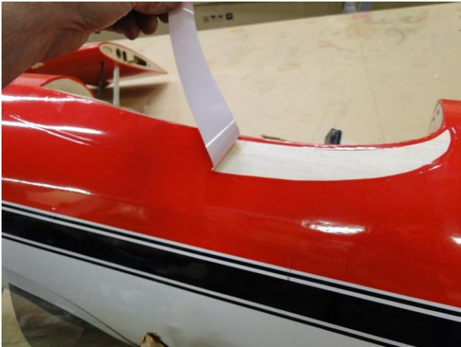
Use a sharp X-Acto Knife to carefully cut away the Covering about 1/16 inch inside the lines. Be careful not to cut the Balsa.
