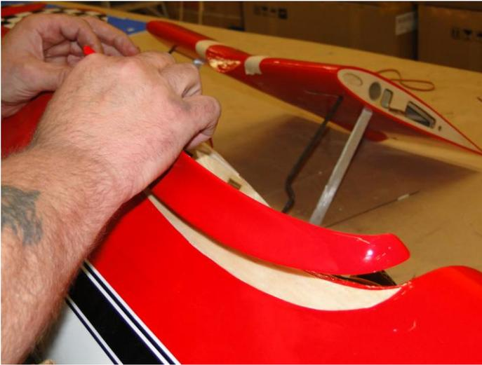
Carefully attach the Fairing. Tape in place until the Epoxy sets up.
