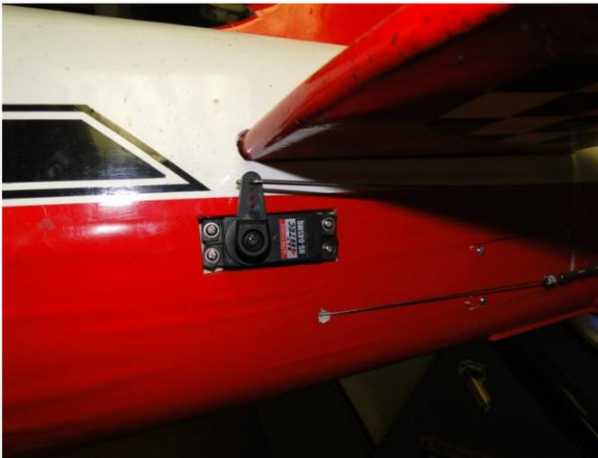
Position the Elevator Servo in the Fuselage and pre-drill the holes using a 1/16 inch Drill Bit. Use the hardware supplied with your Servo for final installation.
