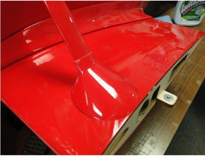
To install the Strut Fairing you will have to cut it back  $\frac{3}{16}$  inch so the non-bent end of the Strut will slide through it. You will have to drill a hole in the top of the fairing to reach the Socket Head Bolt inside. Glue the fairing to the Strut with Hot Glue.
