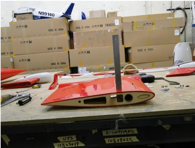
Install the Aluminum Bar in place and use Screws supplied to secure it to the Wing. Sanding off the paint and rounding the corners will help it fit better.
