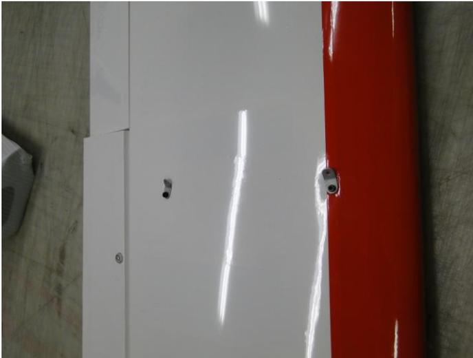
Bend 8 steel straps at a 45° angle. Locate the Blind Nuts on the bottom of the Center and Outer Wings and install Bent Straps using bolts provided.
