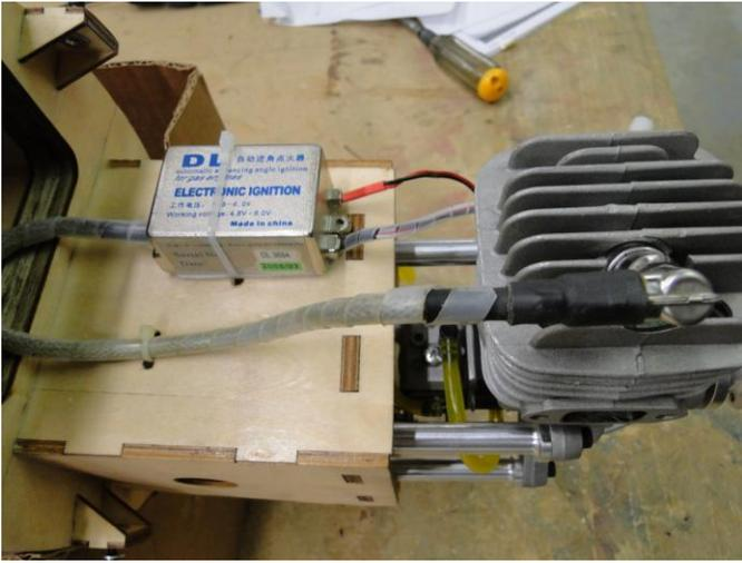
Bottom View of Engine and Ignition Module installed.
