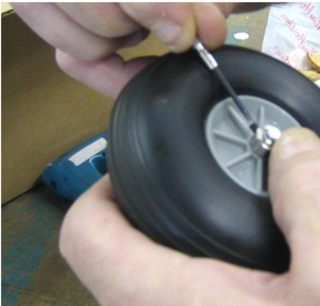
Install one Lock Collar on the Axle where the inside of the Wheel would come to rest.
