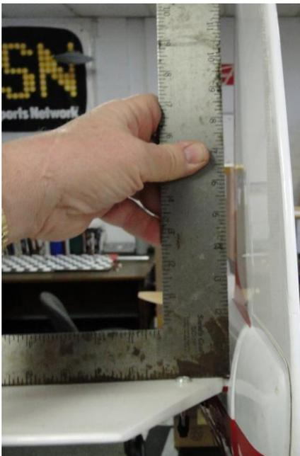
Similar to the Horizontal Stab, cut the Covering on the rear of the Fuselage for the Vertical Fin, insert and mark where to cut away the necessary Covering and use Epoxy Glue to attach.
