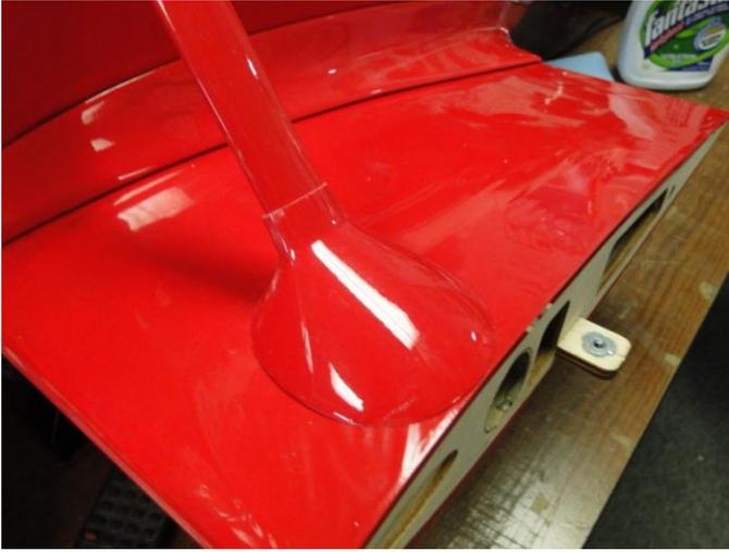
To install the Strut Fairing you will have to cut it back  $\frac{3}{16}$  inch so the non-bent end of the Strut will slide through it. You will have to drill a hole in the top of the fairing to reach the Socket Head Bolt inside. Glue the fairing to the Strut with Hot Glue.
