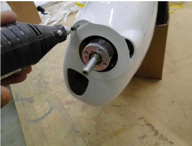
Installing some Engines may require cutting away some of the Engine Box or Fuselage. It is recommended to reinforce any cut-outs and for larger engines.
