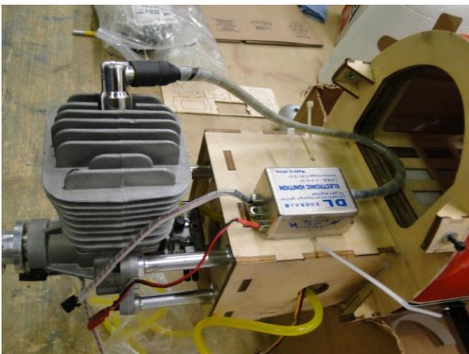
Ignition module is mounted to the bottom side of the engine box.
