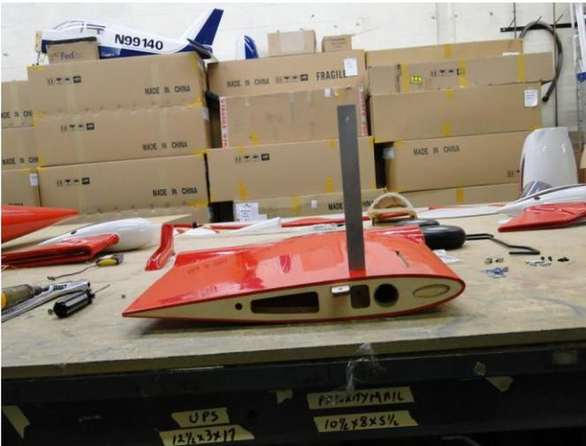
Install the Aluminum Bar in place and use Screws supplied to secure it to the Wing. Sanding off the paint and rounding the corners will help it fit better.
