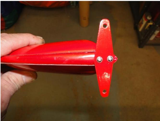
Attach the Rudder Control Horn to the Bottom of the Rudder with 4 Wood Screws provided.
