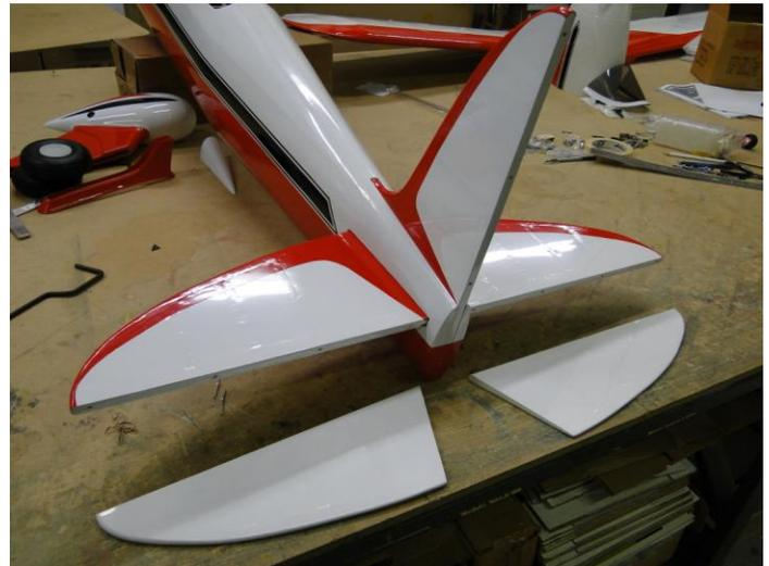
Remove the Elevators and Hinges from the Horizontal Stabilizer and set them aside.
