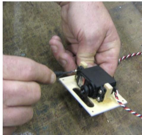
Attach a 12 inch Servo Extension to each Aileron Servo. Tie a nut or small weigh to one end of a light string and drop it through the Wing. Tape or tie the string to the Servo Lead and carefully pull it through the wing. You may be able to get the Flap Servo Lead through the Wing without tying a weight.
