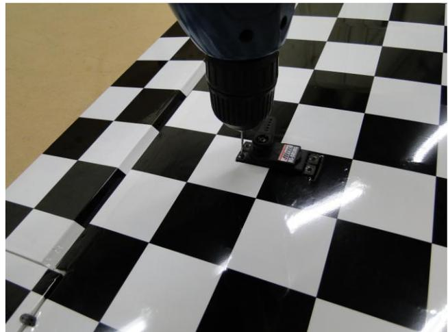
The Flap Servos are mounted to the back of Hatch Covers. Find the openings on the bottom of both Wings and use a sharp X-Acto Knife to cut the Covering. Seal and trim the Covering the same as you have done for the Aileron openings.
