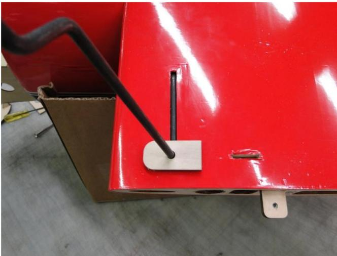
Cut away the Covering on the bottom of the Wings to allow the Wire Landing Gear to mount into the Wing. Slight bending might be necessary.
