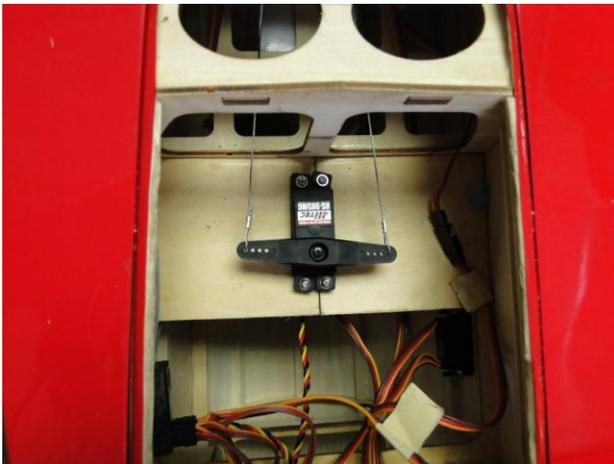
Install the Horns, Clevises and Threaded Couplers onto the Trumpet Bases on the Rudder. With the Rudder Servo Arm in the middle/neutral position and the Rudder in the neutral position (hold in position with Masking Tape), thread a Crimp Fitting over both ends of the Cable and through Threaded Couplers as you did on the Servo Arm. Pull both Cables snug, fold them over and slide the Crimp Fitting into position. Pull both Cables snug, fold them over and slide the Crimp Fitting into position.
