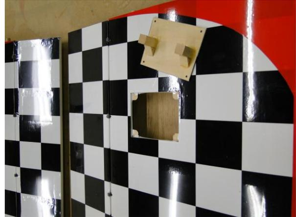
The Flap Hatch Covers do not have cut outs. The screw holes in the Covers and Wing are pre-drilled. You just need to poke a hole in the Covering.
