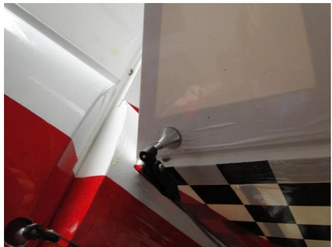
Position the Trumpet Base at the edge of the Elevator beveled edge and 1 inch from the edge closest to the Rudder. Mark the spot and drill a 3/32 inch diameter hole through the Elevator. Install the Trumpet Base with the Trumpet Screw and Washer on the other side of the Elevator. **Do not over tighten.**
