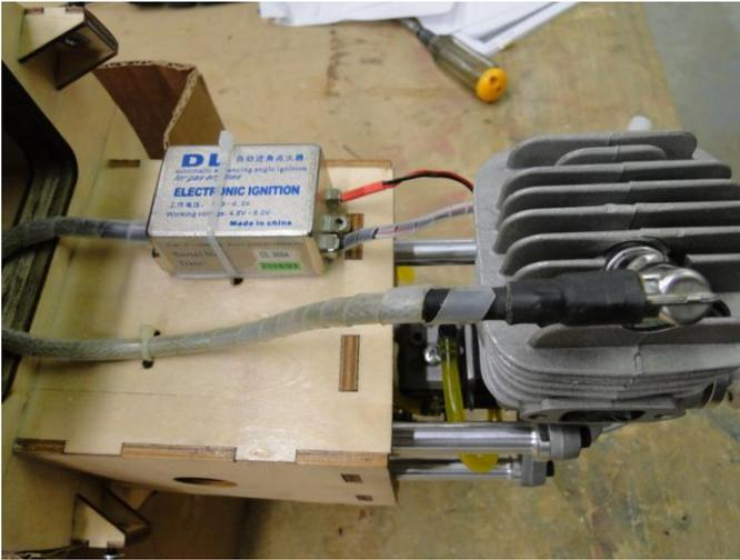
Bottom View of Engine and Ignition Module installed.
