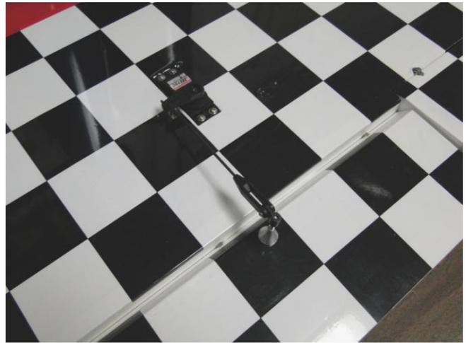
Install the Trumpet Base with the Trumpet Screw and Washer on the other side of the Elevator. **Do not over tighten.**
