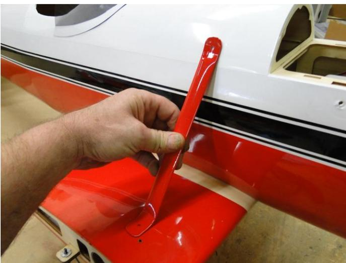
Mount the strut using supplied socket head bolts. Make sure the airfoil shape is pointing forward.
