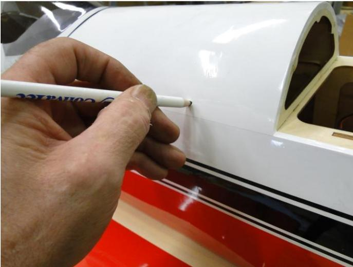
Locate the holes for the strut mount and poke a hole in the covering using a pencil at the fuse and mid wing location.
