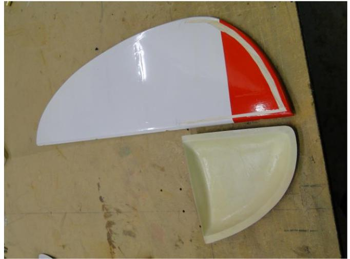
The Rudder comes with Hinges that are pre-installed but not glued permanently. Test fit so that you have 1/16 inch spacing between the Vertical Stab and Rudder. Use Epoxy Glue on the Hinges as you have done before. Remember to make sure they are moving in the proper direction.
