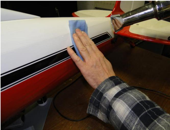
Sometimes in storage or shipping the Covering can sag or wrinkle. Use a small amount of heat from a Heat Gun and a Mitt to go over the entire airplane and smooth any wrinkles in the Covering. Be careful not to use too much heat.
