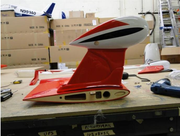
Hold the Wheel inside the upper Wheel Pant and twist to allow the Wheel to slide onto the Axle. This will require you to grind off a minimum of 5/16 inch around the opening of the Wheel Pant. The more you lengthen the opening, the more movement you allow the Landing Gear Wire to flex for rough landings.
