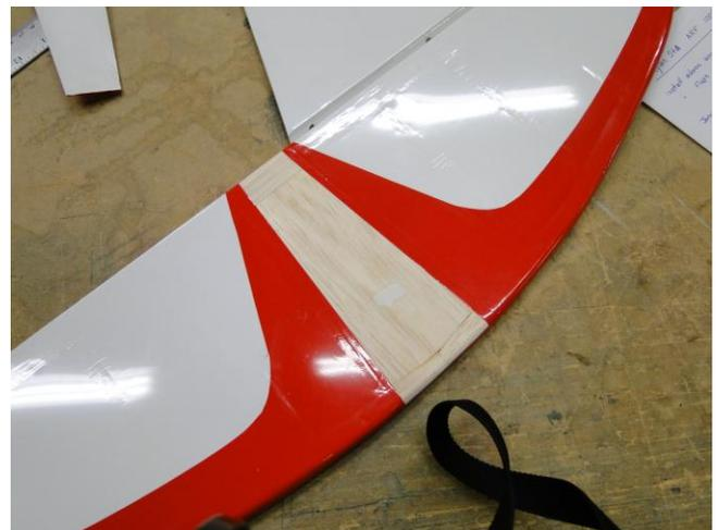
Use a slower bonding Epoxy (like 15 to 30 minute) to attach the Stabilizer to give yourself more time to adjust and clean up.
