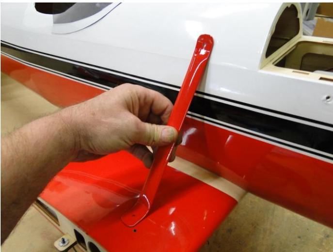
Mount the strut using supplied socket head bolts. Make sure the airfoil shape is pointing forward.
