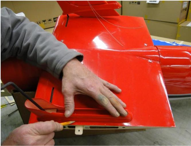
Slide the lower half of the Wheel Pant Assembly over the Landing Gear Wire and push up against the Plywood Wheel Pant Insert and trace around the lower Wheel Pant with a pencil.
