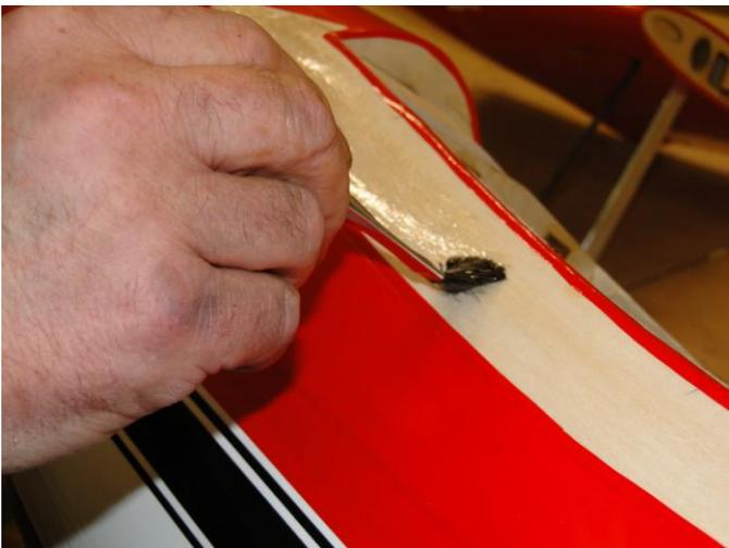
Apply Epoxy to the Fuselage where the Covering has been removed.
