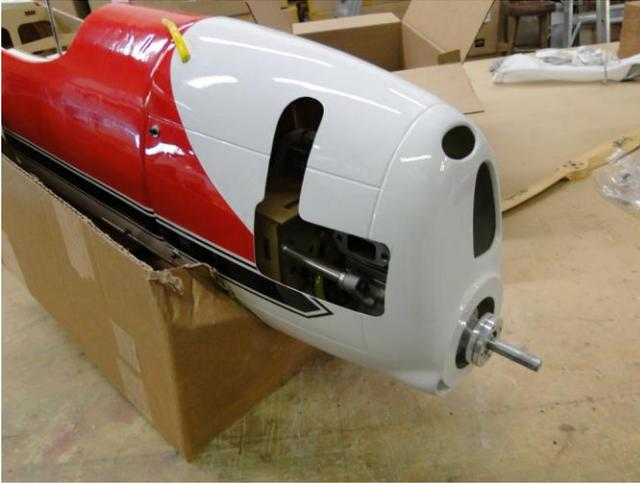
Cut out any the Cowl as needed for your Muffler.
