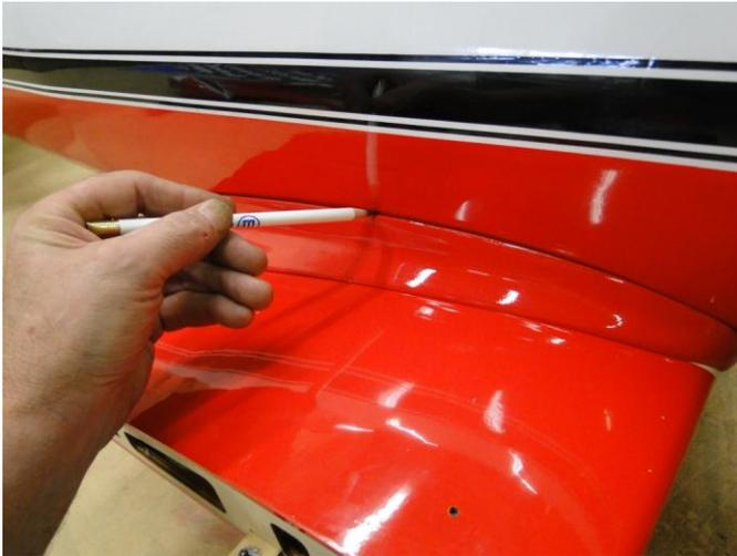
To attach the Fairing to the Fuse side first install the Mid Wing Section with 4 bolts provided (longer ones in front, shorter ones in rear).
