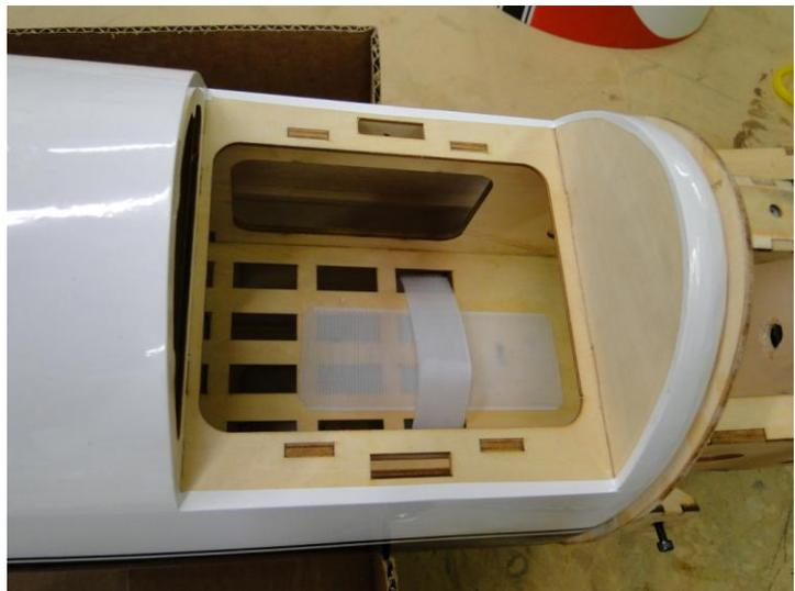
There are many Tank mounting choices but the easiest is to attach Velcro to the top of the Tank, attach Velcro on the inside ceiling of the Fuselage, strap through the vent holes in the front of the Fuselage (we used a Velcro strap) with the Fuel Lines going through the pre-drilled hole in the Engine Box.
