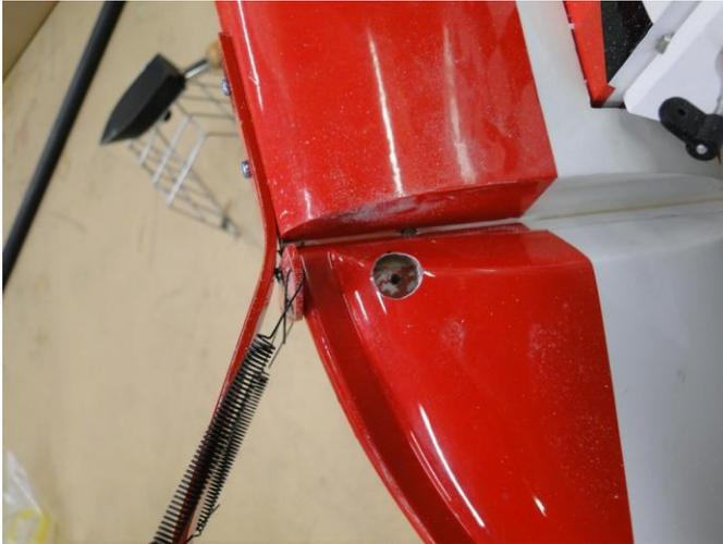
The Rudder has 2 Trumpet Bases that screw together through the Rudder. Position the Trumpet Base at the edge of the Rudder beveled edge and 1 inch from the bottom of the Rudder and mark. Drill a 5/32 inch hole right through the Rudder. Then drill a 1/2 inch hole through the Fiberglass Rudder Cheek on each side.
