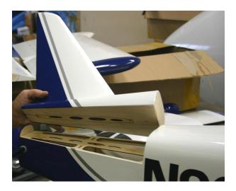
Locate the plastic tubes already installed in the tail block for the rudder pull pull cables (covered over with covering).
