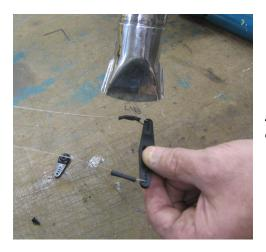
TIP: Use a 3/4 inch piece of 1/8 inch shrink tubing to cover the sharp end of the Cable sticking out of the crimped Joint at both ends of the Cable. You will have to slide this on Cable in advance.
