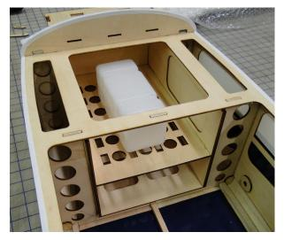
Tip: Stick Velcro to the Fuel Tank and on the Tank Platform for a stronger attachment.
