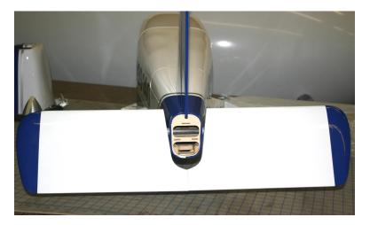
Make sure the Stabilizer rotates smoothly. Sand the portions of the tube that insert into each Stabilizer half to allow the Epoxy Glue to bond well.
