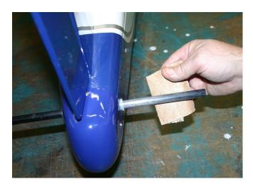
Important: Before glueing the Stab install the Control Horn Bolt with the Bolt pointing <u>DOWN</u>.
