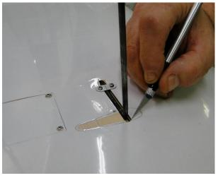
Using a sharp X-Acto Knife cut out the covering approximately 1/16 inch inside the traced line.
