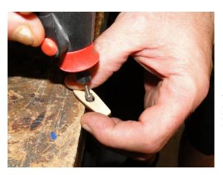
Use a Dremil Tool to elongate the hole in the smaller Fairing Insert so the Fairings won't get ripped off on a rough landing.
