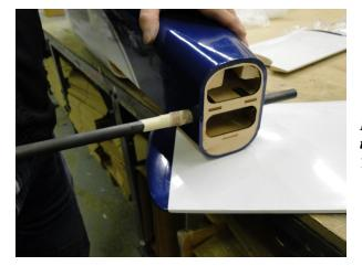
Note: You may have to sand the holes in the Fuselage so the Nylon Bushings sit looser and don't bind the Stabilizer Tube. Slide each half of the Stabilizer into place.
