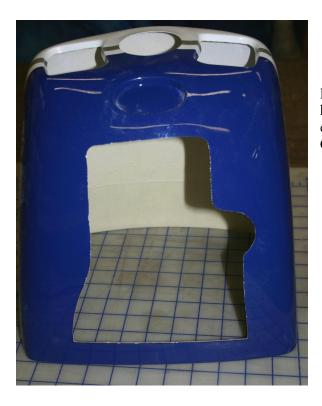
Make the necessary cut-outs in the cowl for the engine you have chosen. Slide the Cowl on the Fuselage so the Prop Shaft exits the center of the Cowl opening and mark the edge of the Cowl on the Fuselage. We suggest using Masking Tape.
