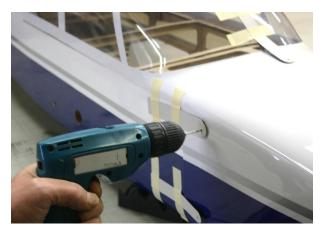
Gently slide the Cowl into place under the tabs (with the engine installed and cut-outs done) up to the Masking Tape marks on the Fuselage. Tape the cowl in place. Drill pilot holes through the center marks with 1/16 inch drill bit. Remove the Card Stock and use Wood Screws to attach the Cowl through the holes you drilled.
