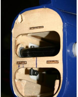
Test fit the new Push Rod to make sure it moves the Stab properly. Make sure it lines up with one of the slots in the plywood surface (that holds the Servo) to allow full movement of the Control Horn.
