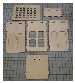
The 6 pieces of the Engine Box are all notched differently to assure correct assembly. Trial fit all the pieces. Sand if necessary. When satisfied, glue all pieces using 30 minute Epoxy Glue. Hold pieces together for a tight fit using clamps.
