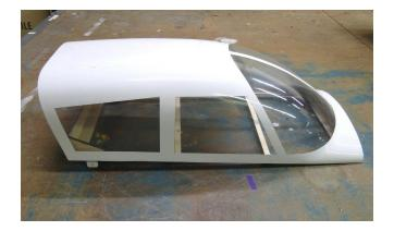
Test fit to see that everything is aligned and seated properly. You may have to sand the front tabs slightly.
