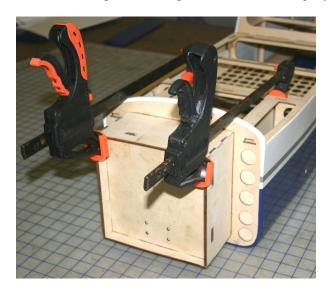
Brace all four sides inside the engine box front with the smaller supplied Tri Stock. Glue the larger Tri Stock to the outside sides of engine block.
