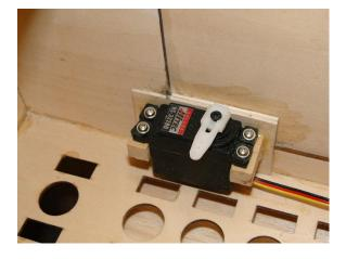
Mark and drill a ¼"hole in the front of the Engine Box to accommodate steering linkage. Just as before, measure a piece of Control Rod with threaded end. Make a "Z" bend on the other end, trim off and attach a Clevis. Use this assembly to connect the Throttle Servo to the Engine Throttle.
