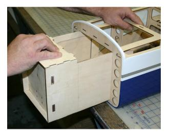
When satisfied, glue box into place with 30 minute Epoxy Glue. Again clamp where able until glue dries.
