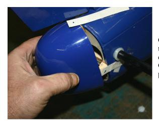
Cut 3 pieces of stiff Card Stock 1 inch x 4 inches and tape them on the Fuselage so that the ends overlap the center of each Wooden Block. Mark these locations on the Card Stock. Gently slide the End Cone into place under the tabs and tape in place.
