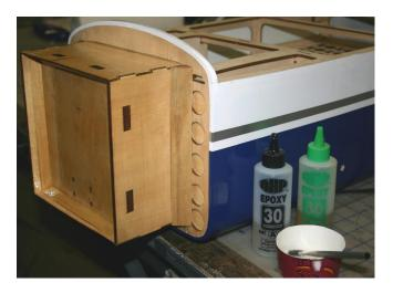
Hint: Mix enough Epoxy Glue to do the job and use a small stiff brush. Use your Heat Gun to warm the glue as you brush it on. The heat will help thin the glue giving a much smoother glass like finish when dry. It also helps the Epoxy Glue soak into the wood easier for greater protection.
