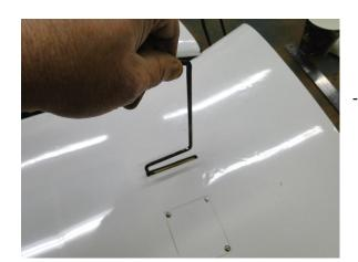
Set in the Landing Gear Struts and position 2 of the Metal Straps and mark the location for the screw holes.
