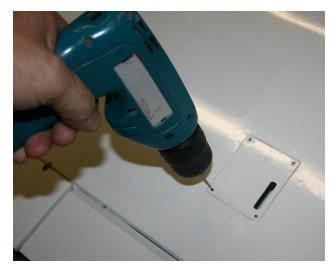
With the hatch cover in place poke a hole in the covering for each screw hole and drill 1/16" holes in the Wing for the Hatch Cover Screws.
