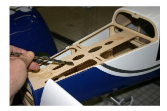
Using same method as with Ailerons, use Epoxy to glue the Rudder Hinges in place.
