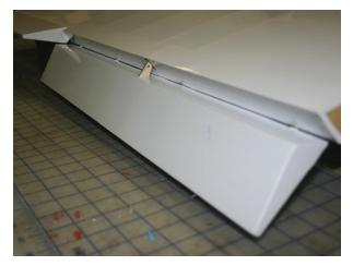
Attach a Clevis to each Flap Push Rods and connect to each Flap Servo Arm with a "Z" bend. Position the Hatch Covers so the Push Rods goes through the hole in the trailing edge of the Wing and connects with the Flap Control Horn (already installed). Secure both Flap Servo/Hatch Assemblies to the wing using 4 Small Wood Screws using the same procedure as the Aileron Servo Hatch Covers.
