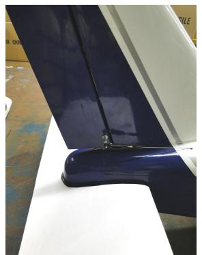
Position the Trumpet Base at the edge of the Rudder beveled edge and 1 inch from the bottom of the Rudder and mark where to drill a 5/32 inch hole through the Rudder. Install the 2 Trumpet Bases with the Trumpet Screw. **Do not over tighten.**
