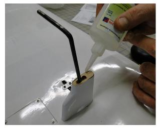
Slide the Fairing into place and glue to the bottom larger Insert and the top smaller Insert.
