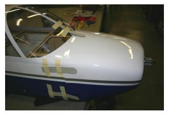
Cut 5 pieces of stiff Card Stock 1 inch x 4 inches and tape them on the Fuselage so that the ends overlap the center of each Wooden Block and mark that location on the Card Stock.
