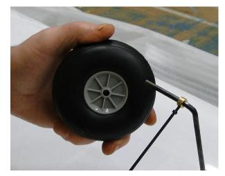
Slide a Wheel Collar onto each Landing Gear Strut. Slide the Wheel on and then another Collar. With the Wheel centered in the middle of the Strut tighten the Wheel Collars just tight enough so the Wheel turns freely.
