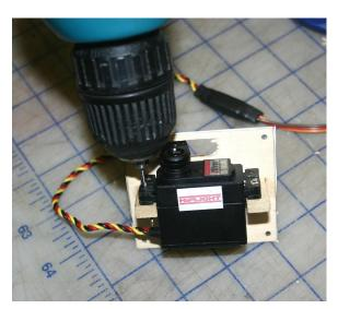
Position the Aileron Servos so the Servo Arm exits the middle of the Hatch cut out. Pre-drill the holes in the Mounting Posts with a 1/16 inch Drill Bit. Attach Servos to the Hatch Cover Mounting Posts using the hardware supplied with your Servos. Do the same for the Flap Servos.
