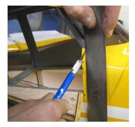
Colored Vinyl Trim (¾ inch wide) has been included to stick around the Side Door opening to close the gap between the Fuselage and Canopy and to cover up any chipped paint. First clean the inside of the door frame to help it bond better. Then draw a fine line with a sharp X-Acto Knife 1/8 to ¼ inch around the Door opening and peel away the paint.
