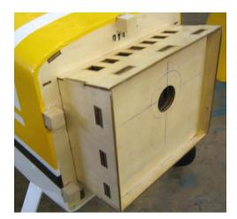
Use Epoxy Glue to attach the 5 Hardwood Blocks around the edges of the Fuselage Firewall, 2 on each side and 1 on top. Locate the 2 lower Blocks so they miss the raised section on the lower sides of the Cowl.
