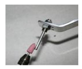
TIP: You may have to remove burrs from the Axle using a Dremil Tool so that the Lock Collars will easily slide over the Axle Shaft.
