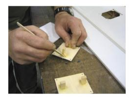
Position the Aileron Servos so the Servo Arm exits the middle of the Hatch cut out. Pre-drill the holes in the Mounting Posts with a 1/16 inch Drill Bit. Attach Servos to the Hatch Cover Mounting Posts using the hardware supplied with your Servos. Do the same for the Flap Servos.
