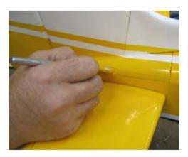
Use a sharp X-Acto Knife to remove the Covering from both sides of the Fuselage where the Rudder Pull-Pull Cables exit.
