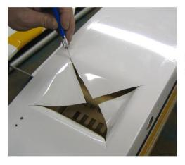
Use a sharp X-Acto Knife to cut the Covering from corner to corner in the first panel on the bottom of the fuselage.
