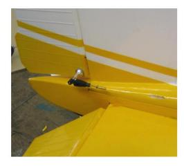
Install the Horns, Clevises and Threaded Couplers on the Trumpet Bases on the Rudder.
