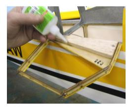
Press the window into the Window Frame. Be careful not to get any glue on your fingers or the windows. If using Canopy Glue you should tape into place while the Glue dries.
