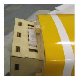
There are many Tank mounting choices but the easiest is to attach Velcro to the top of the Tank, attach Velcro on the inside ceiling of the Fuselage, strap through the vent holes in the front of the Fuselage (we used a Velcro strap) with the Fuel Lines going through the pre-drilled hole in the Engine Box.
