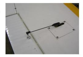
Attach a Clevis to each Flap Push Rods and connect to each Flap Servo Arm with a "Z" bend. Position the Hatch Covers so the Push Rods goes through the hole in the trailing edge of the Wing and connects with the Flap Control Horn (already installed). Secure both Flap Servo and Hatch assembly to the wing using 4 Small Wood Screws.
