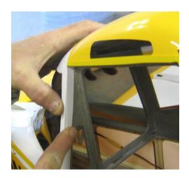
Use Epoxy Glue to mount the Hinges into the Side Door frame. Check for proper direction of the Hinge movement. When dry, trial fit the Door on the Fuselage before glueing the Hinges into the Fuselage with Epoxy Glue.
