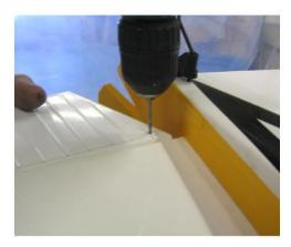
Position the Trumpet Base at the edge of the Elevator beveled edge and 1/2 inch from the edge closest to the Rudder. Mark the spot and drill a 3/32 inch diameter hole through the Elevator. Install the Trumpet Base with the Trumpet Screw and Washer on the other side of the Elevator. **Do not over tighten.**
