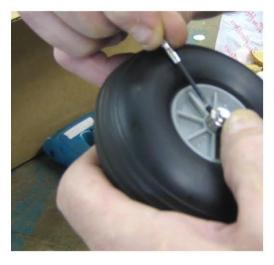
Slide on the Wheel and an Axle Collar and tighten the Collar Set Screw so the Wheel spins freely.
