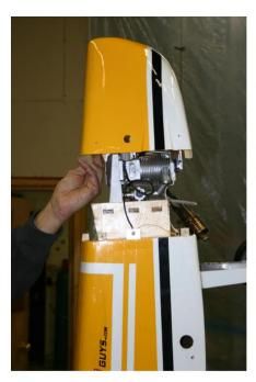
Your Engine will have to be positioned on the Engine Box so that the prop shaft exits the centre of the Cowl opening. It works best to stand up the fuselage. It can be held that way in a work bench or with the landing gear supported by a step ladder.
