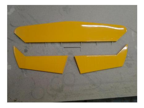
Position the Elevator halves so there is a 1/16 inch gap at the outer edges of the Stabilizer. Mark the location of the Elevator Joiner on each Elevator and drill 5/32 inch holes at the marked locations. Test fit the elevator halves. If they are not in alignment remove and bend the elevator joiner. Use Epoxy Glue to attach the Stabilizer Joiner like you did for the Tail Wheel Arm into the Rudder and then glue the Elevator Hinges also using Epoxy.
