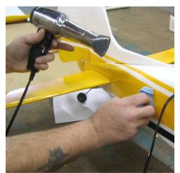
Sometimes in storage or shipping the Covering can sag or wrinkle. Use a small amount of heat from a Heat Gun and a Mitt to go over the entire airplane and smooth any wrinkles in the Covering. Be careful not to use too much heat.
