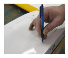
Place the Hatch Cover in position and mark the location of the 4 holes with a pen or pencil.
