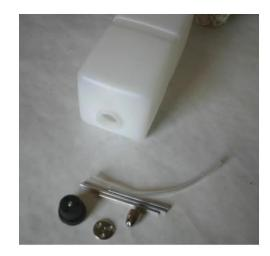
Using the supplied hardware, assemble the Fuel Tank. Carefully, bend the metal tubing to avoid kinking. You might need to use a larger size Fuel Tubing for your engine.
