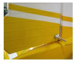
Cut the Cable into 2 equal lengths and thread the Cable through these new uncovered holes in the rear of the Fuselage. Thread one Crimp Fitting over the end of one Cable, then thread the Cable through the outer hole in the your Large Rudder Servo Arm. Fold back the Cable 1 inch and slide the Crimp Fitting over the Cable end. When satisfied with the fit, crimp the fitting. Repeat for the other end of the Servo Arm with the other Cable.
