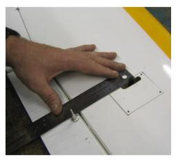
Secure both Aileron Servo and Hatch assemblies to the wing using 4 Small Wood Screws. The Servo Arms are on opposite sides of the Hatch Covers. Then position the Trumpet Base at the beveled edge of the Aileron and align with the Aileron Push Rod and mark the location. Drill a 3/32 inch diameter hole on these marks.
