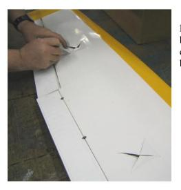
Find the openings for the Aileron and Flap Servos on the bottom of both Wings and use a sharp X-Acto Knife to cut the Covering, from corner to corner. Seal and trim the Covering the same as you have done before.
