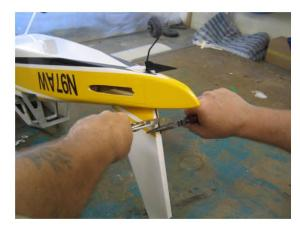
Insert the completed Tail Wheel Assembly through the Tail Wheel Bracket as far as it will go. Use a pair of Vise Grips and Pliers to bend the portion of the Tail Wheel Arm coming through the top of the Fuselage about 1 inch above the Fuselage.
