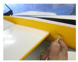
If installing the Servos in the rear of the Fuselage find the location for the Elevator Servo(s) and use a sharp X-Acto Knife to cut the Covering, from corner to corner. Seal and trim the Covering the same as you did for the Fuselage Hatch Cover
