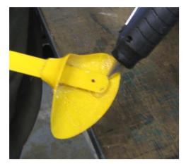
Use Silicone or Hot Glue to hold the Cuff in position on the end of the Strut.
