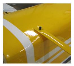
With the Wing Strut airfoil facing forward, bolt the end of the Wing Strut through the pre-drilled hole into the Wing using a  $6-32 \times 5/8$  inch Socket Head Bolt. Mark where to drill a 9/64 inch hole in the other end of the Strut at the pre-installed Blind Nut in the Fuselage. This may be already done at the factory.
