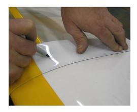
Trace around each Middle Wing Fairing with a pencil on the Wing and remove the Covering where the Fairing makes contact with the leading edge of the wing sheeting. Use an X-Acto Knife like you have done before. Be careful not to cut the Balsa but you can roughen up the Balsa (scratch with X-Acto) and plastic Fairing (use Sandpaper) to make a better bond. Attach the Fairings with Epoxy Glue and tape into position until they dry.
