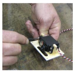
Attach an 18 inch Servo Extension to each Aileron Servo. Using a light string, tie a nut or small weigh to one end and drop it through the Wing Rib opening until it appears in the Aileron Hatch opening. Tape or tie the string to the Servo Lead and carefully pull it through the wing. You may be able to get the Flap Servo lead through the Wing without tying a weight.
