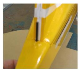
Find the 1/8 inch hole at the rear of the Vertical Fin and the matching hole on the bottom of the Fuselage. Punch a hole in the Covering and push the Tail Wheel Arm through from the bottom.
