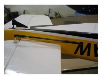
The installation of the Control Horn and Clevis on the Trumpet Base is the same if you are using an Elevator Pushrod.
