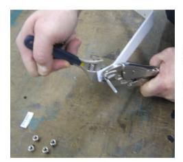
Secure the 2 Axles to the Main Landing Gear using the Axle Nylock Nuts
