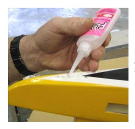
TIP: Remove the screws and add a drop of Thin CA Glue to each hole and re-attach the Tail Wheel Bracket. This will help harden the Balsa and stop the Wood Screws from loosening.
