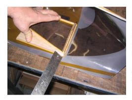
If you are installing the Side Door, position it on the inside of the Canopy with the bottom corner of the window cutout of the Door matching the window painted on the Canopy. Mark the outside edge of the door with a pencil or fine tip marker.
