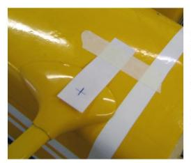
Fasten the other end of the Struts in place with a  $6-32 \times 5/8$  inch Socket Head Bolt. Tape a piece of heavy paper over the top bolt and mark the location of the Bolt. Slide the Strut Cuffs to rest against the Fuselage (under the paper) and mark the location on the Cuffs where to drill a  $\frac{1}{4}$  inch hole.
