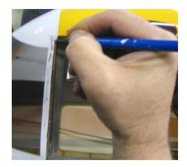
Apply the Vinyl Trim overlapping the untouched paint by 1/16 inch and folding into the Door opening. Trim to fit.
