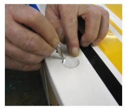
Locate and cut holes in the Covering on both sides of the Fuselage for the Wing Tube (1 inch), Wing Bolt (1/4 inch), Servo Leads (9/16 inch) and Dowel (1/4 inch).
