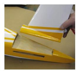
Attach the Vertical Fin with Epoxy Glue. 5 Minute Epoxy would be best but anything up to 30 Minute Epoxy will be suitable.
