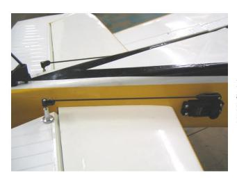
Install the Control Horn and Clevis on the Trumpet Base as you did for the Rudder. Thread the Elevator Push Rod into the Clevis and make a "Z Bend" in the other end to install through your Elevator Servo Arm.
