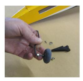
Slide one Lock Collar over horizontal Axel portion of Tail Wheel Arm. Then slide on the Tail Wheel. Position the Wheel so it is in line with the vertical portion of the Tail Wheel Arm. Tighten the Set Screw in the first Lock Collar with it pressed up against the Wheel. This may be already done for you at the factory.
