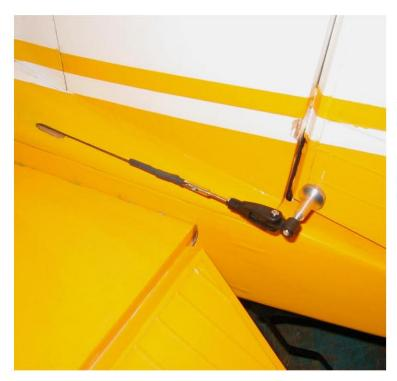
When satisfied with the lengths, carefully crimp the Cable fittings and trim the excess Cable.
