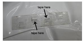
Attach the 4 clear fin holders with fins to the balloon by peeling the adhesive tape backing and sticking them approx 10" from the rear of the balloon.
