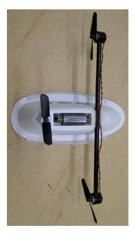
You will need to balance the balloon neutral (won't float up or down). In order to do this you will need to add some washers, pennies or plasticine (ballast) inside the gondola. Untie your string to the balloon and re-adjust the ballast until correct. The more accurate the balance, the easier the blimp will fly.
